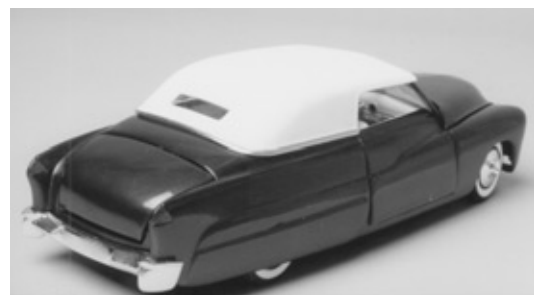
The great looking, and carefully fitted, taillights were carved from a clear red toothbrush handle.
