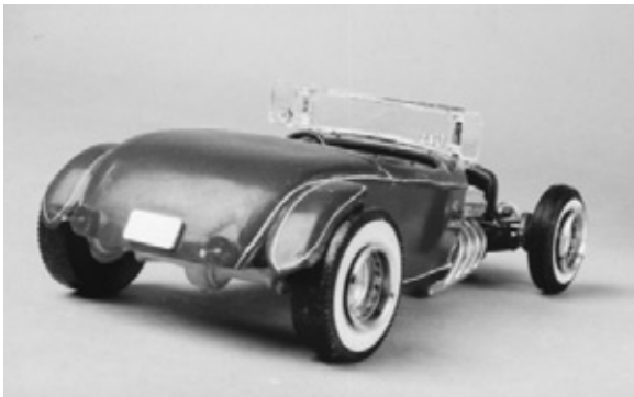
Check out the rake, the molded rumble seat, custom taillights, abbreviated fenders and painted undercarriage. Note how the old tires have shrunk away from the old AMT rims.
