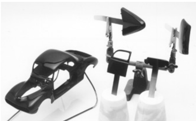
The beautiful candy Brandywine lacquer finish was then applied over the fogged base color. Note that all the parts were painted separate from the body. Rick is a master painter.
