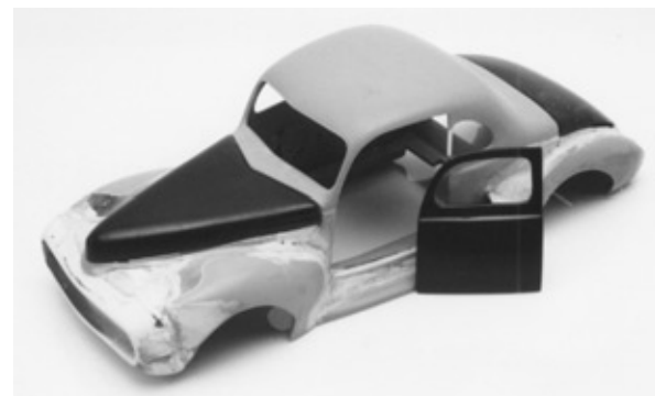
The original model was in remarkably good condition, but it needed to be redone. The original driver's door was replaced, but used to match the paint. Note the excavated original bodywork.
