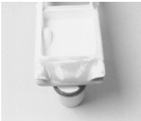
Just the front and back customized areas were treated to spray primer (ever notice how many of the details of early-era customs were obliterated by too-thick paint?). After drying (the cure time wasn't much different from modern acrylic lacquers), I sanded the surface using 400 grit sandpaper (again, no modern sanding sticks were used).
