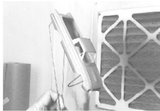
After deciding that the customized areas were ready for paint, a thin coat of AMT lacquer primer was applied to the entire model, allowed to dry, and then the model was mounted on a coat hanger. The AMT metallic green was then applied, first to the recessed areas, and then along the bottom, along the sides, and then on horizontal surfaces.
